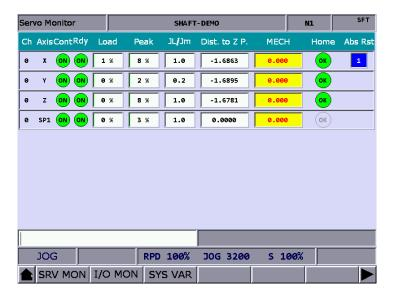
(3) Set the system to JOG or MPG mode to use the absolute reset function. In JOG or MPG mode, move the axis to the position to be defined as the origin, enter "1" and press **ENTER** to complete the setting. Meanwhile, the Home indicator is on, meaning that this axis has completed homing.
